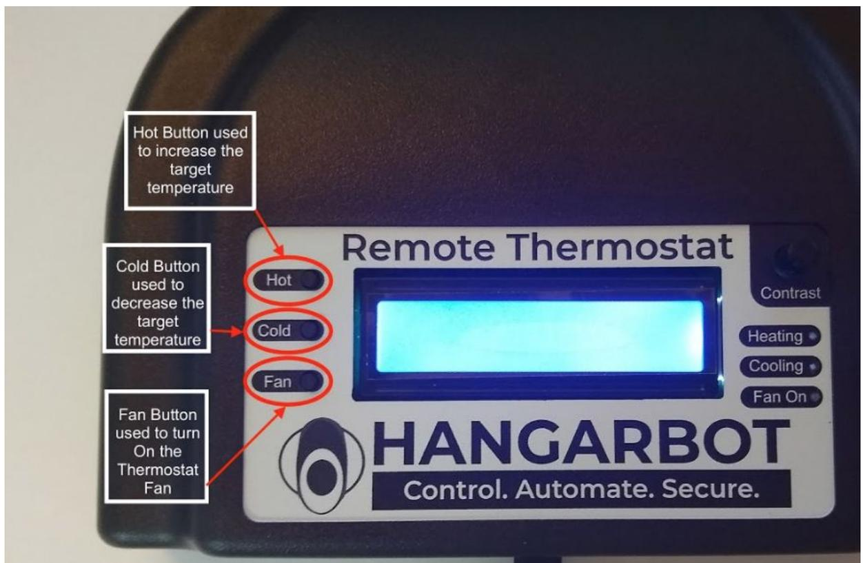
Figure 10 Hot/Cold/Fan buttons for manual control of the Thermostat
