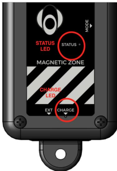
**Figure 1 Door Sensor LED indicators**
